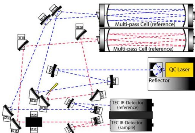
FIGURE 1 Optical setup of the QCLAS
