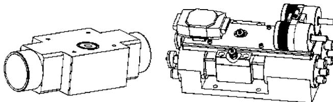
FIGURE 2 The cell-body design and the compact, thermally coupled reference/sample cell assembly with the temperature and pressure sensors mounted at the top
