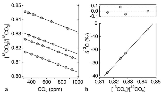
**FIGURE 4** (a) Dilution curves of four calibration gases with different CO<sub>2</sub> isotopic composition. (b) Comparison of relative isotope ratios determined by QCLAS with the δ-values measured by IRMS
