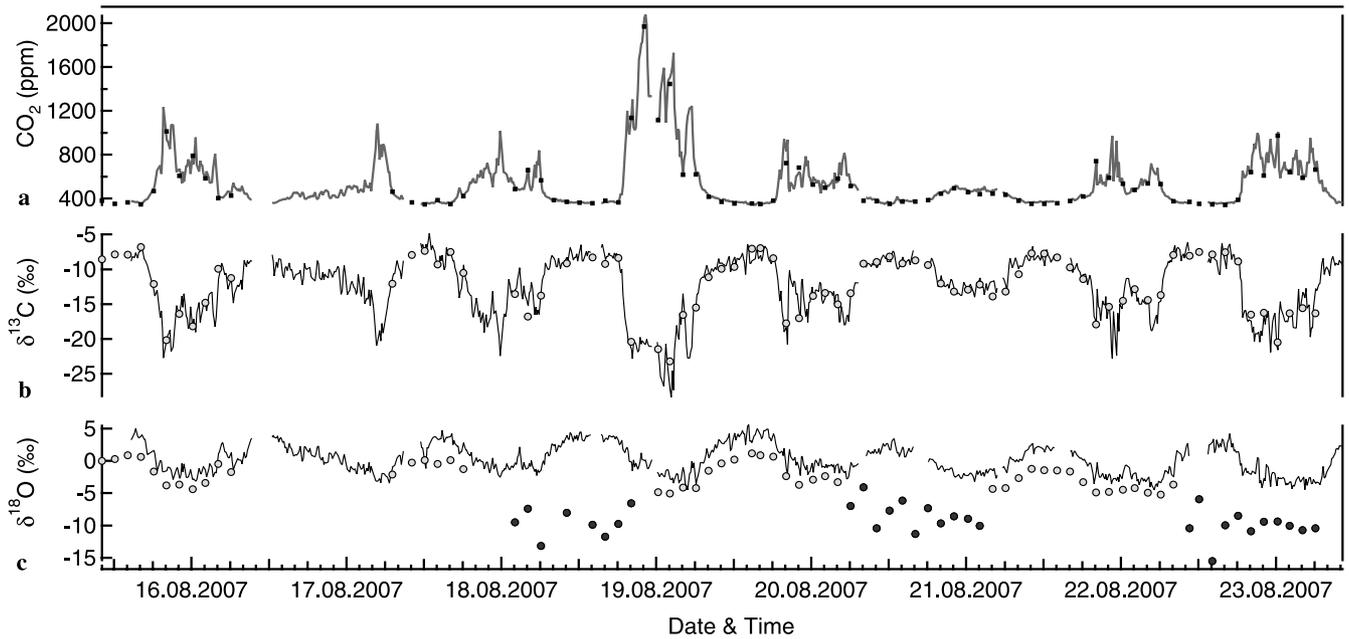
**FIGURE 5** (a) Time series of the carbon dioxide mixing ratio measured by the QCLAS (line) and with an IRGA (dots). The corresponding  $\delta^{13}\text{C}$  and  $\delta^{18}\text{O}$ -values measured by the laser spectrometer are shown in (b) and (c). For comparison IRMS  $\delta$ -values are also given. The closed symbols for the  $\delta^{18}\text{O}$ -values indicate sampling issues with the metal flasks (details in text)
