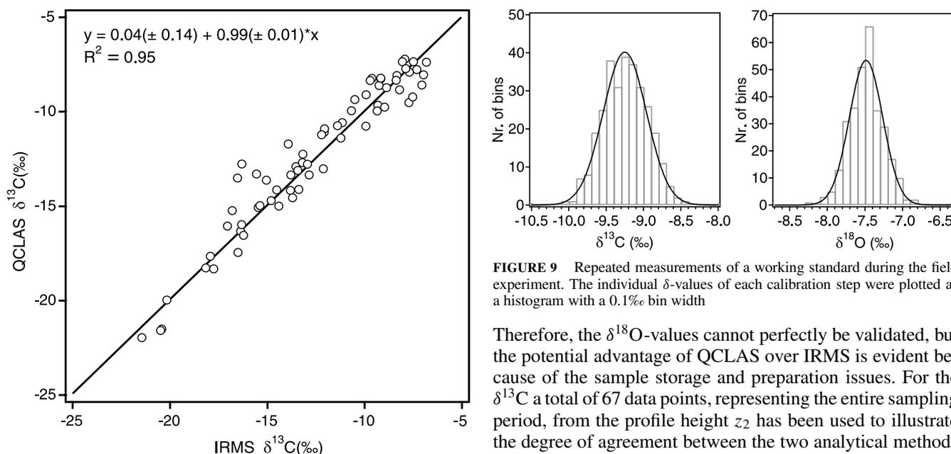
**FIGURE 8** Comparison of  $^{13}\text{C}$ -values measured with QCLAS and IRMS. Flask samples for the IRMS were collected every 2 h during the experimental period (August 15–23, 2007). The linear regression indicates an excellent agreement between the two techniques
