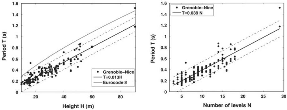
**Fig. 3** First resonance periods of RC shear wall buildings in Grenoble and Nice (France) (*black dots*) versus their height (*left*) and their number of levels (*right*), the linear regression (*solid black line*) and the 95% confidence interval (*dashed black lines*). The solid grey line is the Eurocode 8 formula with  $C_t = 0.05$
