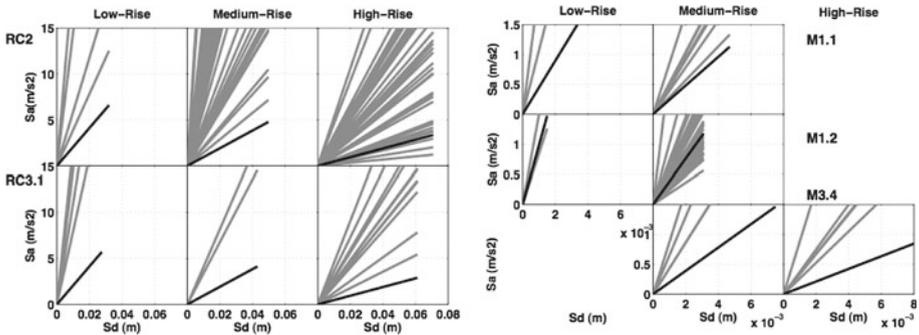
**Fig. 4** Elastic part of the experimental capacity curves obtained from all the structures in Grenoble (grey) compared to Risk-UE curves (Lagomarsino and Giovinazzi 2006) (black) for different height classes. **a** RC buildings (RC2=shear walls, RC3.1=infilled frames). **b** Masonry buildings (M1.1=rubble stone, M1.2=simple stone, M3.4=simple stone with concrete slabs)
