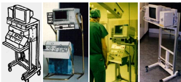
Figure 4: Design process, sketch, model (1:10), working model (1:1) and the product - The Monitor-Frog.
