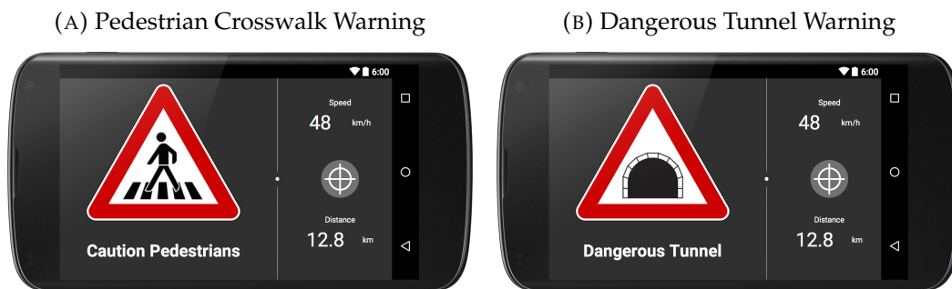
FIGURE 3.13: Two examples of the in-vehicle warning intervention shown to drivers approaching an accident hotspot
