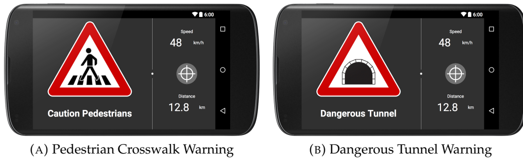
FIGURE 4.3: Two examples of the in-vehicle warning intervention shown to drivers approaching an accident hotspot
