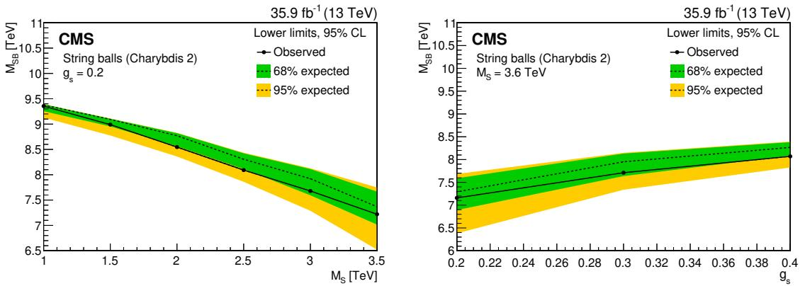
**Figure 11.** The 95% CL lower limits on a string ball mass as a function of the string scale  $M_S$  for a fixed value of the string coupling  $g_s = 0.2$  (left) and as a function of the string coupling  $g_s$  for a fixed value of the string scale  $M_S = 3.6$  TeV (right). The inner (outer) band represents the  $\pm 1$  ( $\pm 2$ ) standard deviation uncertainty in the expected limit. The area below the solid curve is excluded by this search.
