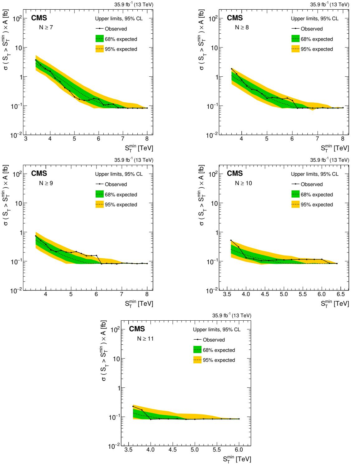
**Figure 7.** Model-independent upper limits on the cross section times acceptance for five sets of inclusive multiplicity thresholds,  $N \geq 7, \dots, 11$  (left to right, upper to lower). Observed (expected) limits are shown as the black solid (dotted) lines. The inner (outer) band represents the  $\pm 1$  ( $\pm 2$ ) standard deviation uncertainty in the expected limit.
