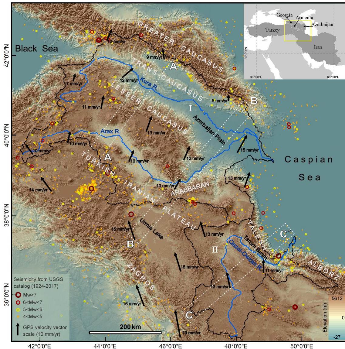
Fig. 2.1: Topography of the Turkish-Iranian Plateau and Caucasus Region from a SRTM 90m DEM (Jarvis et al., 2008). Yellow Square in inset includes the study area. Black arrows: GPS velocity vector respect to stable Eurasia reference frame (Reilinger et al., 2006a). Colored circles: seismicity of the area based on USGS earthquake catalogue. Black polygons: studied rivers catchment boundaries discharging to the Caspian Sea: (I) Kura-Arax and (II) Qezel-Owzan. White dash-lines: swath profiles location (A–A', B–B', C–C' and D–D' displayed in Fig. 2.3).
