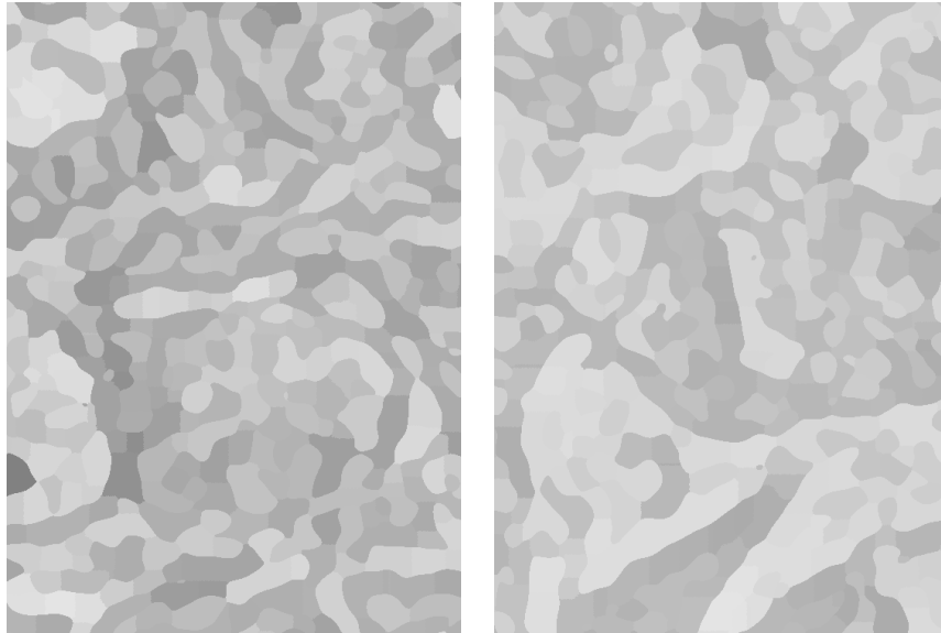
Figure 4.6: Zoomed in to fig. 4.1. Images filtered with are Log Gabor filter with a larger spatial constant followed by a two sided watershed to create region pixels. The image provides mean pixel intensity of the super pixels.
