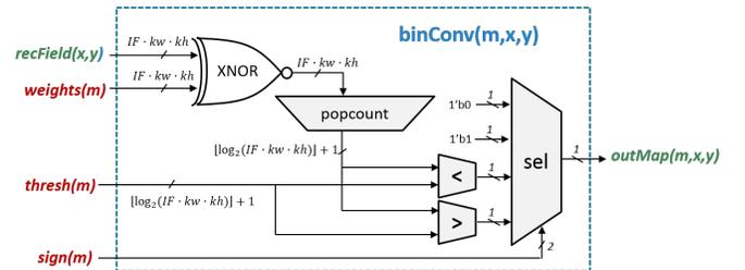
Fig. 2. Hardware architecture of the combinational building block for computing binary convolutions. Every  $\text{binConv}(m, x, y)$  module instantiated within a convolutional layer produces the binary value of the output neuron at location  $(x, y)$  of the  $m$ -th output feature map.
