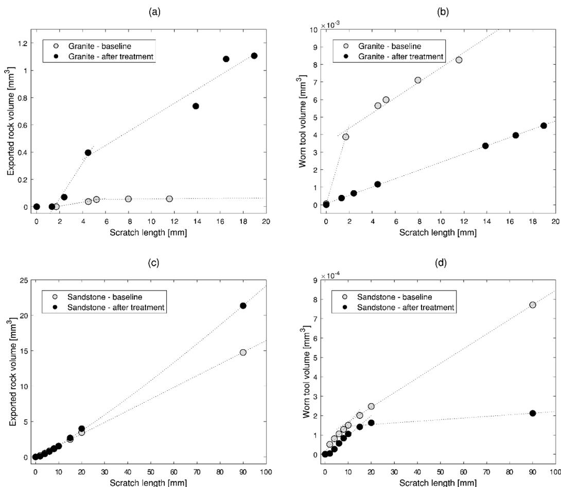
**Fig. 1: Removed rock volume and worn tool volume after scratching experiments on a granite (a) and (b); and a sandstone (c) and (d) for the untreated material case (gray circles) and after the thermal treatment (black circles).**
