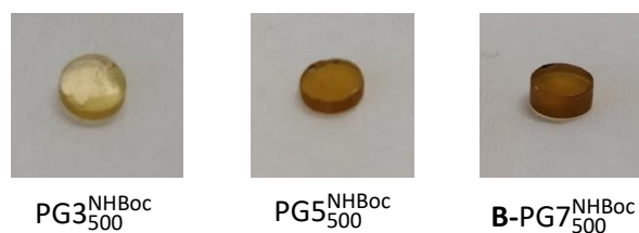
Figure 5-1: photographs of typical DP pills after vacuum annealing; the bulk DP samples tend to have a darker color with increasing g .
