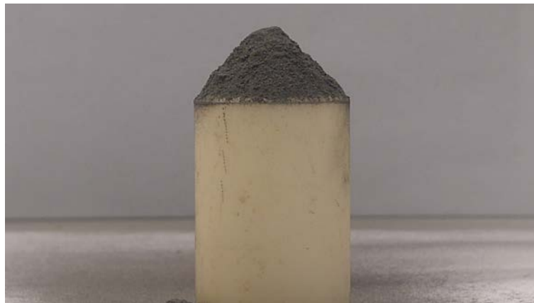
Figure 11: Angle of repose measurement for sample 1.
