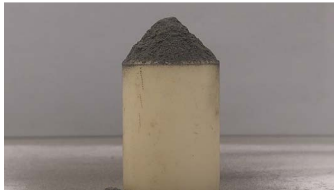
Figure 6: Example of the angle of repose measurement for sample 1.
