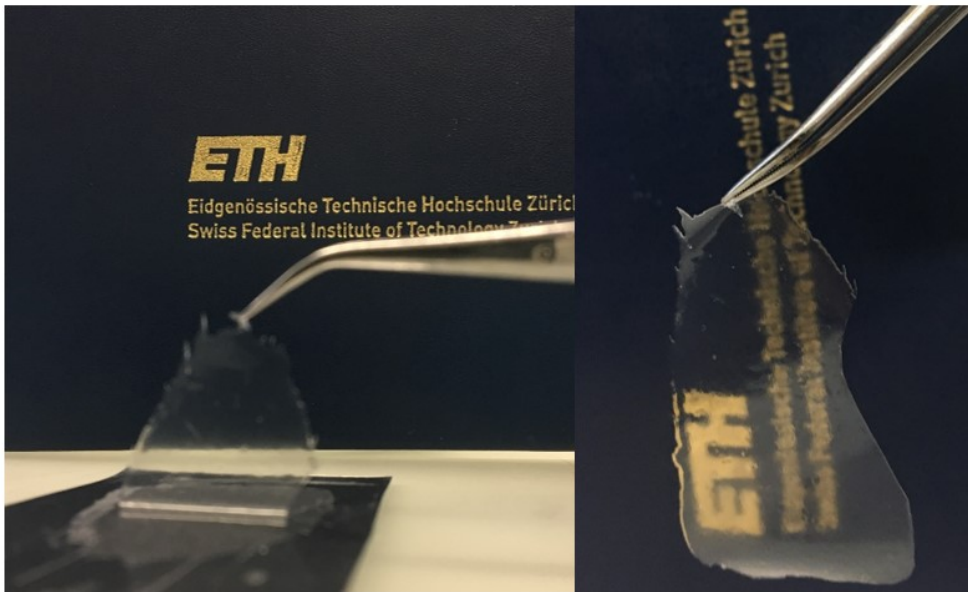
Figure 4.3: Freestanding, transparent, 50 \mu\text{m} thick PCIL membrane formed via hot-pressing.
