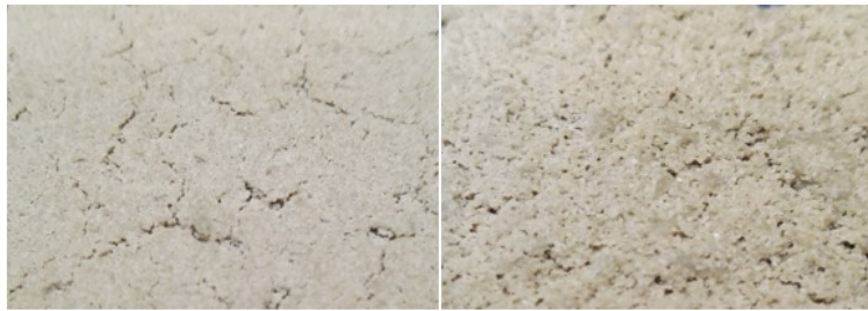
Figure 8.7: Cement-based membrane obtained with polymer h (left) and i (right), after spray drying.
