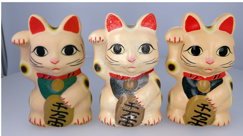
Figure 4.7: Our replica of the cat model (right) has a superior surface quality to that created with a ZCorp 650 powder printer [3ds16] (left) or hydrographic transfer [PDP + 15] (middle).
