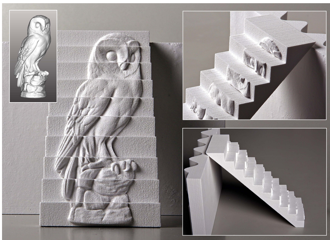
Figure 3.2: Inspired by street artwork painted over the steps of a staircase, we use our algorithm to embed a 3D model of an owl into a staircase. Constrained to a thin layer, the relief does not affect the function of the staircase, while being much more resistant than paint to erosion and aging.
