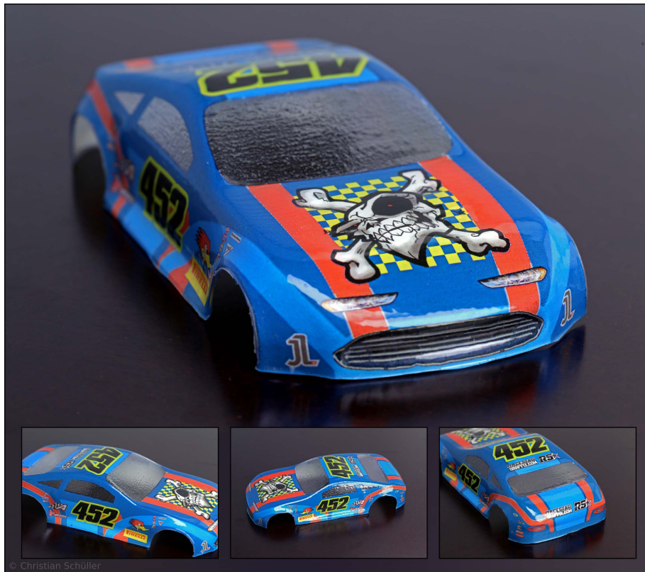
Figure 4.12: An RC car shell fabricated with our method using transparent plastic.
