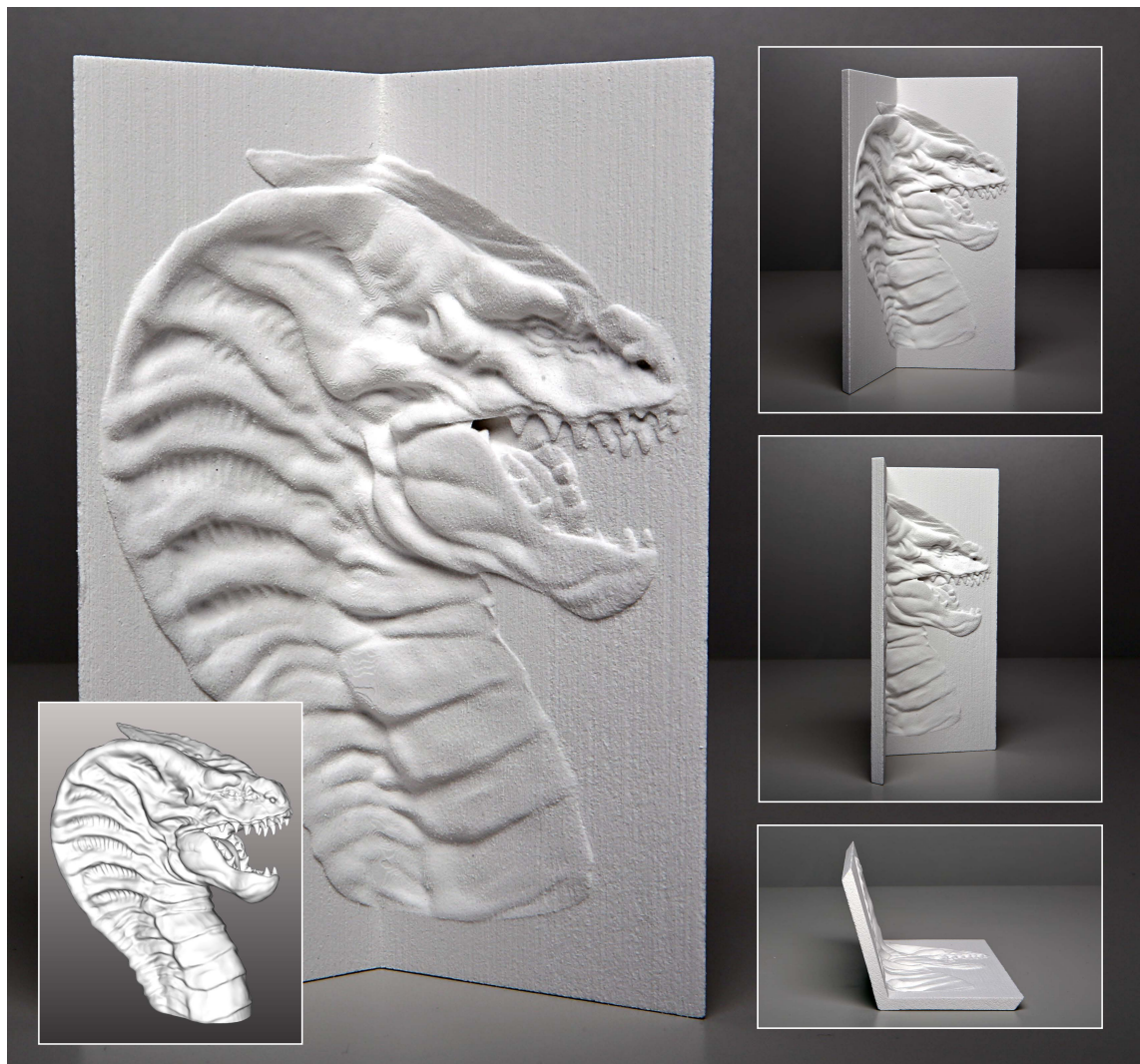
Figure 3.3: Appearance-mimicking surface of the Dragon Head model constrained to carve a V-shaped, thin geometry.
