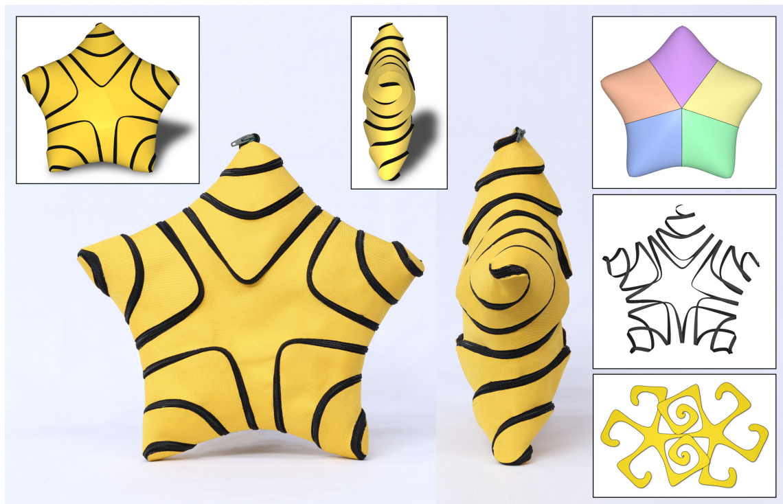
Figure 5.2: The star model fabricated with our fastening rig. The insets on the left and in the middle show the developable model from a front and side perspective. Note how the fabricated star perfectly resembles the predicted shape. The segmentation is shown in the top right corner; below it a visualization of the zipper tape and the flattened zippable. The physical result has a height of 27 cm.
