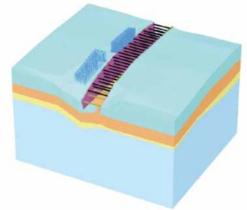
Fig. 9 Excavation test case—Deformation analysis of an earth-retaining structure
