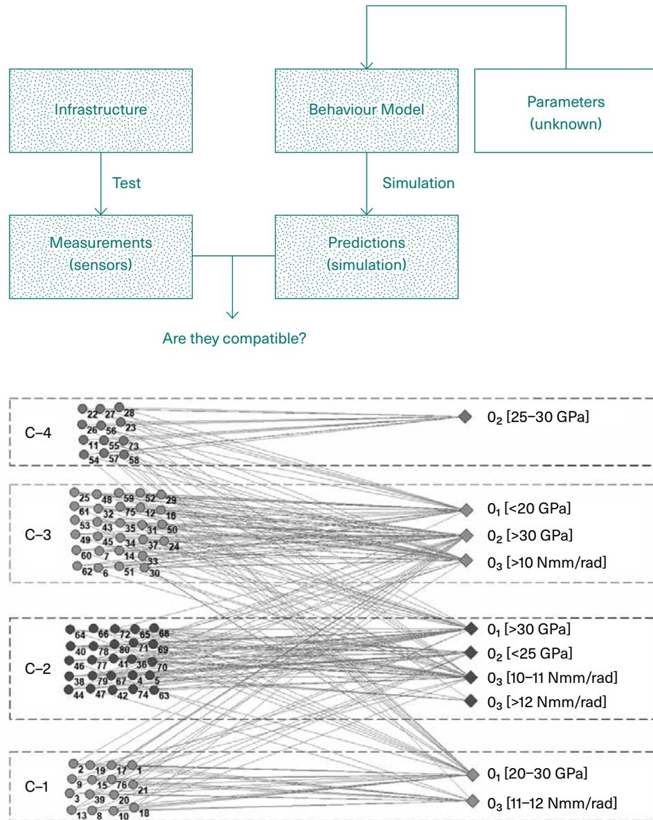
Fig. 7 EDMF methodology to identify good model-parameter values
