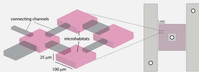
Fig. 2. Schematic view of the chip containing 364 connected microhabitats of dimensions 100 X 100 X 25  $\mu\text{m}$ . The connecting channels are 15  $\mu\text{m}$  deep and 15, 30 or 60  $\mu\text{m}$  wide. Microhabitats are connected to side reservoirs by nanoslits
