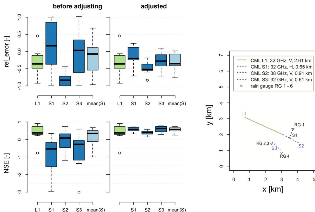
Fig 1: Relative error (top) and Nash-Sutcliffe efficiency index (bottom) evaluated on one long CML (L1), three short (S1-S3) CMLs, and mean rainfall from the three short CMLs (mean(S)). Performance statistics is evaluated for each of the 13 rain events. Adjusted rainfall estimates (right) have substantially higher NSE than before adjusting (middle). Experimental layout of four CMLs and five RGs (right).
