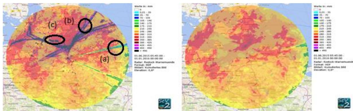
Figure 1: Radar data correction shown on the example of the Rostock/Warnemünde radar. The left panel shows the DX-product from the German weather service accumulated over 6 months before corrections. Three major problems can be observed: beam blockage (a), non-meteorological echoes along shipping routes (b) and non-meteorological echoes at fixed locations (c). The panel on the right shows the same data after correction.
