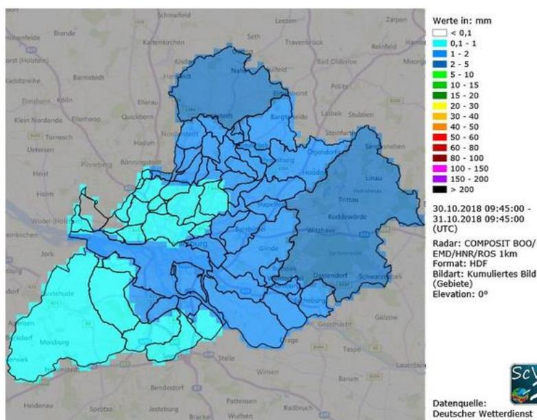
Figure 3: Map as part of the operational test platform for WaBiHa within Stuck, showing the rainfall amount for the past 24 hours for each catchment.
