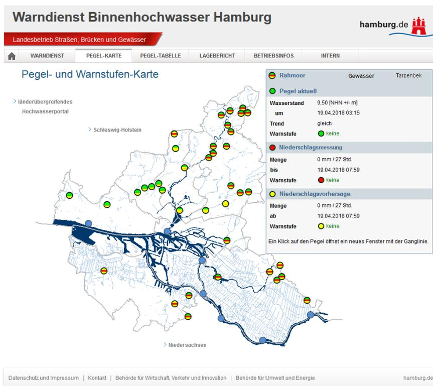
Figure 2: Map as part of the operational test platform for WaBiHa within StucK. Shown are the three-part warning symbols at each water level gauge location and an info box that provides more detailed information for one selected water level gauge location.
