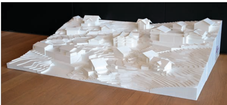
The architectural planning model for a new construction site at Krattigen village. Removable plot and variants of the new building. Dimensions: 90x60x20 cm. Scale: 1 : 200.
