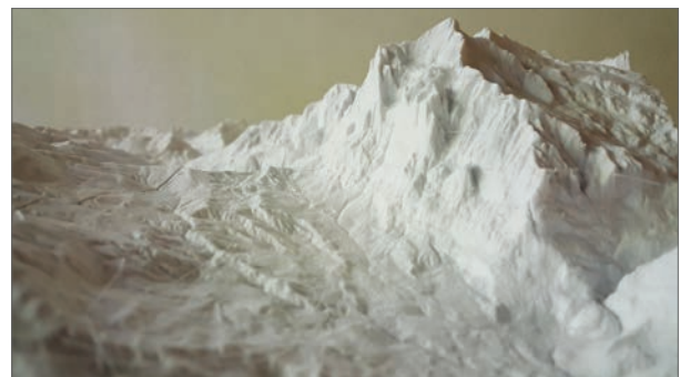
Detail of the canton Bern relief, showing “Mount Wetterhorn” from the west. Raw 3D printed tiles before clean-up.
