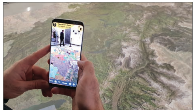
Figure 3: Augmented Reality: Overlaying Geodata and references to Spelterinis areal imagery on a 6.25 x 4 m Orthophoto in the Swiss National Library.
