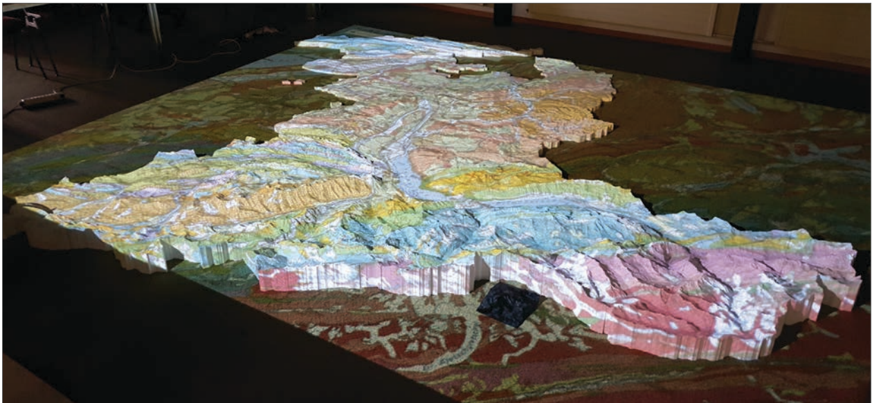
Canton Bern – 3D printed Terrain Model, 1 : 25,000. Dimensions: 494 x 456 x 17 cm. 360 Tiles, each 19 x 19 cm. Overlay: map.geo.admin.ch showing the "Geological map of Switzerland 1 : 500,000" by swisstopo.
