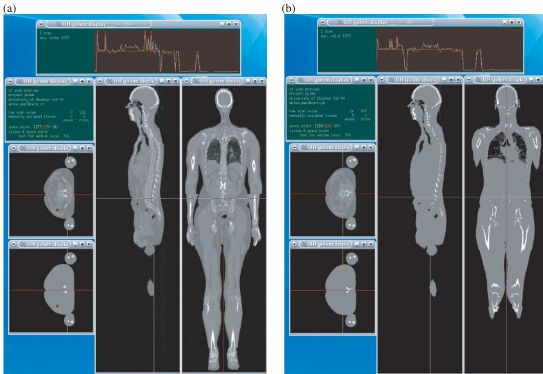
Figure 1. Screen shots are presented of the software tool developed to assess the performance of the tissue assignment algorithm. (a) A slice from the ‘Golem’ CT-scan, where the raw density values are displayed on a linear brightness scale as pixels. (b) The result of filtering this image with the simple threshold algorithm. Note the histogram tool that displays the raw data across the slice and the values from the algorithm superimposed.
