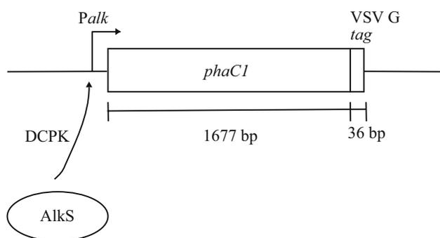
**Fig. 1** *phaC1* expression from plasmids pET702 (not to scale). The expression of *phaC1* from the *PalkB* promoter is positively regulated by the AlkS polypeptide in the presence of an inducer such as DCPK
