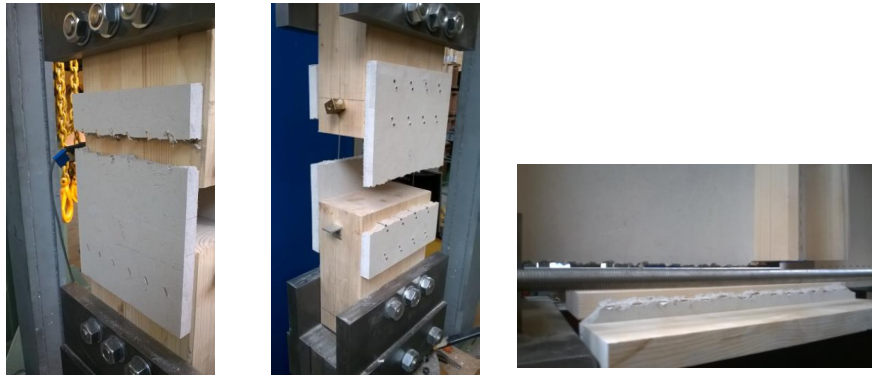
Fig. 3.39: Failure of GFB in tension and in shear during the testing campaign, as reported in [70]
