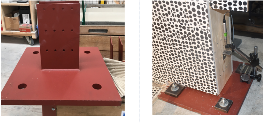
Fig. 3.7: Hold-down device consisting of two slotted-in steel plates and 12 dowels with d = 8\text{mm} (left) and an edge stud during testing (right)
