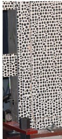
Fig. 5.25: Hysteresis of the shear wall, sheathed with one side with GFB, under cyclic loading with introduced IDR according to the Figure 5.24 and corresponding damage pattern and damage intensity
