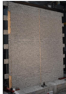
Fig. 5.23: Hysteresis of the shear wall, sheathed on both sides with GFB, under cyclic loading with introduced IDR according to the figure 5.22 and corresponding damage pattern and damage intensity
