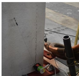
Fig. 5.23: Hysteresis of the shear wall, sheathed on both sides with GFB, under cyclic loading with introduced IDR according to the figure 5.22 and corresponding damage pattern and damage intensity
