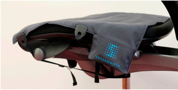
Fig. 1. Textile pressure mat (sensomative science) fixed with two textile straps and belt loops at the seat pan of an office chair.
