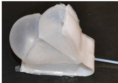
Figure 2.5: Rotary Soft Pneumatic Actuator. Reprinted from IEEE/RSJ International Conference on Intelligent Robotics , pp. 442 – 458, Yi Sun, Yun Seong Song, Jamie Paik, Characterization of silicone rubber based on soft pneumatic actuators , 2013, with permission from IEEE. © 2013, IEEE [8].
