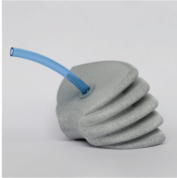
Figure 1.1: The realized 3D-printed inflatable rotary actuator.
