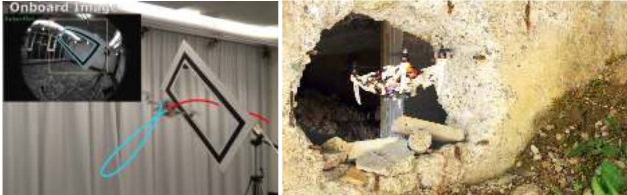
Figure 5: Aggressive drone flight through narrow gaps can be achieved with dynamic trajectories and active vision (left) (Falanga et al., 2017). A target application for this approach would be to enable a flying robot to enter structures such as earthquake-damaged buildings through small apertures in an emergency response (right) (Falanga et al., 2018).
