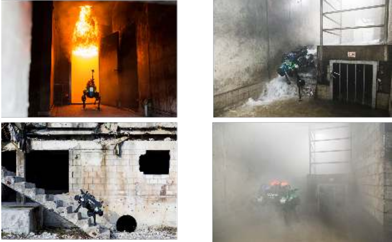
Figure 2: Modular quadrupedal robot ANYmal being deployed in challenging disaster environments (Hutter et al., 2017), highlighting its ability to navigate over rough terrain and in degraded sensing conditions, and demonstrating its resistance to fire and water.
