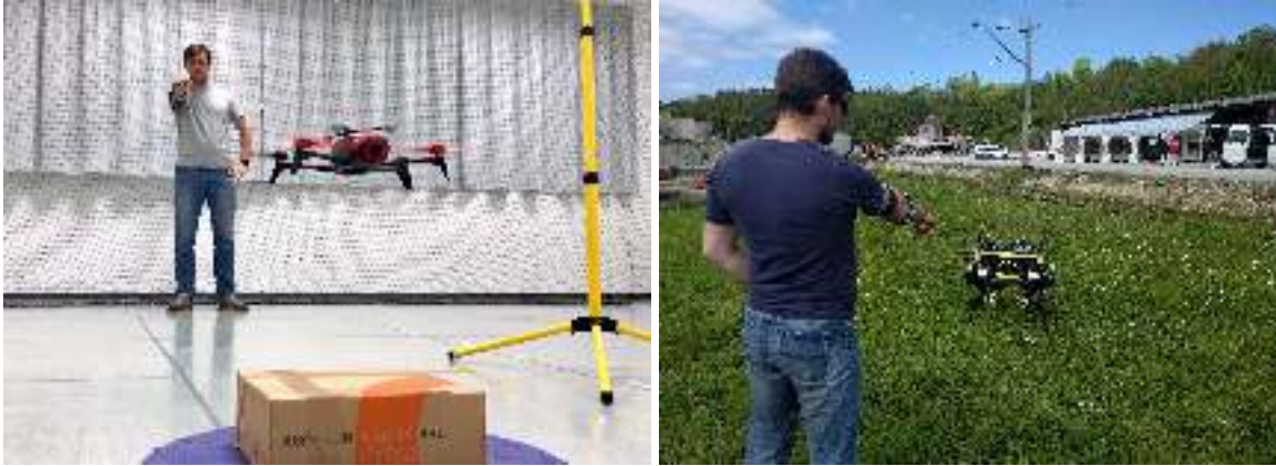
Figure 10: Human-robot interface from (Gromov et al., 2016; Gromov et al., 2018), in which the operator uses pointing gestures, estimated from sensors worn in armbands, to provide navigation commands to both flying and legged robots.
