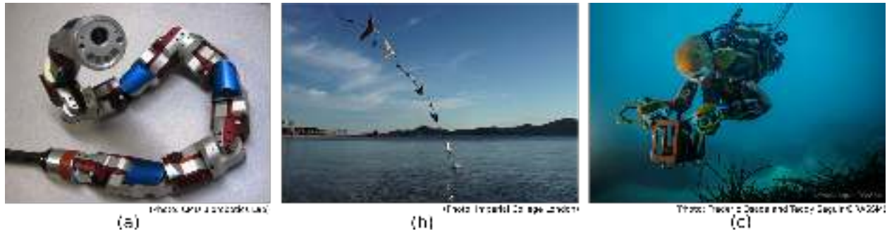
Figure 8: Examples of novel robot morphologies with applications to rescue robotics: (a) snake robots can maneuver into small spaces (Wright et al., 2007), (b) hybrid aerial-aquatic robots can perform surveys in littoral environments (Siddall and Kovač, 2014), and (c) the OceanOne embodied ROV offers an intuitive avatar for underwater manipulation (Khatib et al., 2016).
