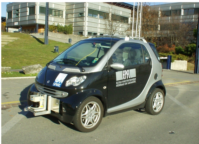
Fig. 1. Our autonomous Smart car platform at EPFL. The white SICK laser range finder used for mapping and obstacle detection can be seen attached to the front of the vehicle. The camera used for lane detection is mounted below the rear-vision mirror inside the car (and is attached to the yellow/light-gray cable).
