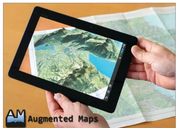
Figure 2: Prototype of a mobile Augmented Reality Application for the extension of traditional paper maps.
