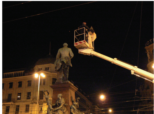
Figure 2. Pointcloud acquisition by laser scanning of the Alfred Escher statue on a cherry picker.
