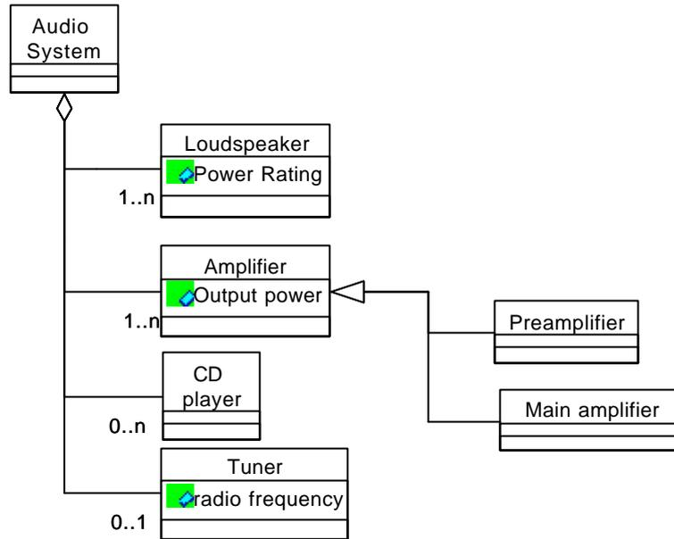
Figure 2. A generic structure for an audio system
