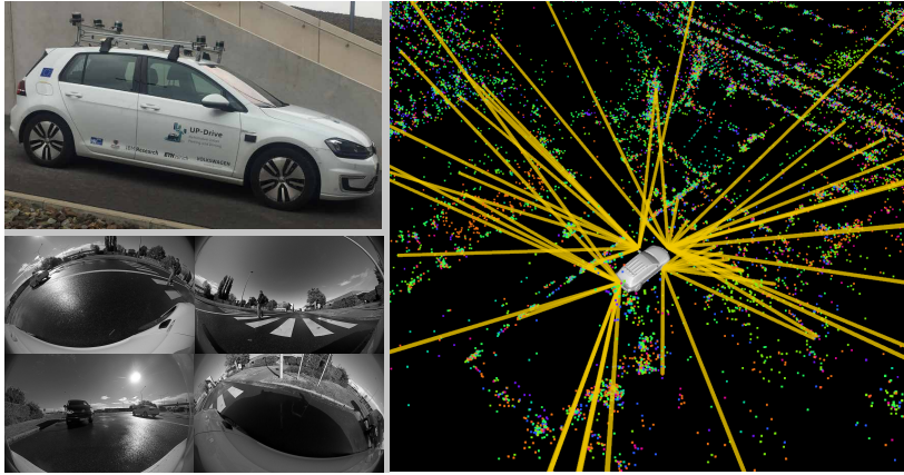
Figure 7.1: We aim at accurately localizing the UP-Drive vehicle depicted in the upper-left corner in a map of visual features depicted on the right side. Features are extracted from images of the surround-view camera system (lower-left corner) and matched against 3D landmarks in the map. Inlier matches, centered on the estimated 6DoF pose of the vehicle in the map, are illustrated as dark yellow lines on the right side.
