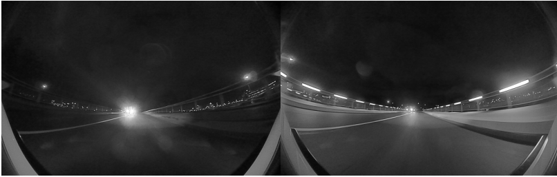
Figure 7.7: On the left, a sample image of a trajectory segment that fails to localize at night. A lack of structure and street lighting renders it unfeasible to match a sufficient number of map landmarks. A few meters later, street lighting is present (right side), and localization is picked up again.
