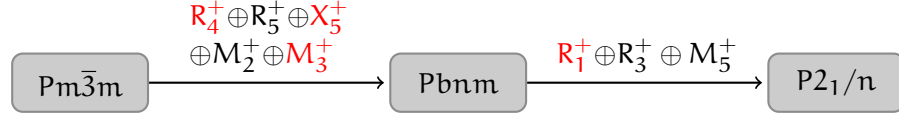
Figure 9: Subsequent symmetry lowering of the cubic perovskite structure due to lattice distortions. Starting from cubic undistorted \text{Pm}\bar{3}\text{m} the symmetry gets first lowered to \text{Pbnm} , which is the nickelate high temperature metallic structure. During the MIT the symmetry gets further lowered to \text{P}2_1/\text{n} in the low temperature regime of nickelates. The important non-negligible distortion amplitudes are highlighted in red.
