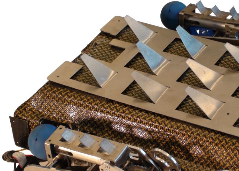
Fig. 4. Close-up view of the scaled plates under the main body and shanks that dug deep into the loose soil and stably supported the robot, even in the steep slopes of the simulated crater.
