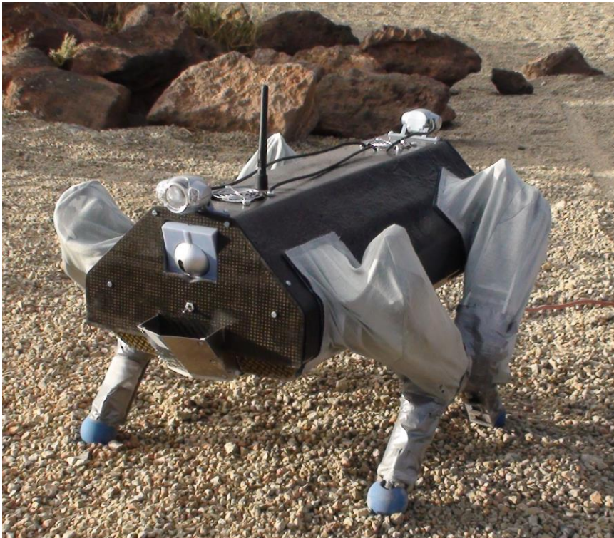
Fig. 1. The ALoF robot during the ESA Lunar Robotics Challenge. In addition to its basic configuration it was equipped with pan-tilt cameras, lights, a dust-protection cover, and scaled plates under the shanks and the main body.
