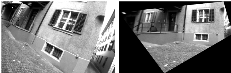
Figure 4.2: An example of an orthophoto (on the right) generated automatically by the proposed framework for the corresponding original image shown on the left, by estimating a local mesh illustrated in Figure 4.3.
