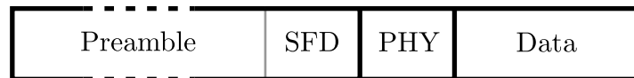
Figure 2.4: A DW1000 UWB packet is separated into three portions: 1. The synchronization header, consisting of preamble and start frame delimiter (SFD) sequences, enables receiving modules to synchronize to the transmission; 2. The physical header (PHY) is used to transmit the packet’s length and datarate, and is additionally used to mark the transmission and reception timestamps; and 3. the packet data, which additionally includes a two-byte Reed-Solomon error-correction code. Further information is available in [11].
