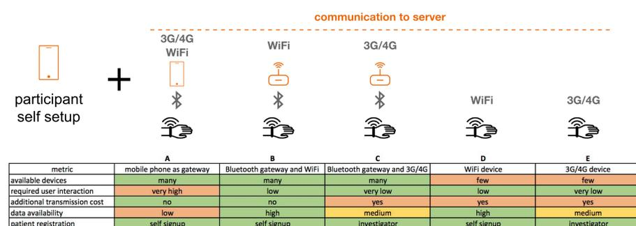
**Strategies for end to end connectivity:** It can be differentiated between devices that require a gateway to communicate with the internet (A, B, C) and those that are able to establish a direct connection (D, E). The best strategy depends on the specific tasks, the participant group, type and amount of data to be transmitted as well as the geographic setting and available devices. A, B and C were used in different projects, a trial with setup D is in planning.
