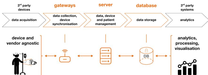
**How it works:** A gateway collects data when device is in reach and exchanges information with a database. The system is device agnostic so 3<sup>rd</sup> party applications and systems can be used at both ends.
