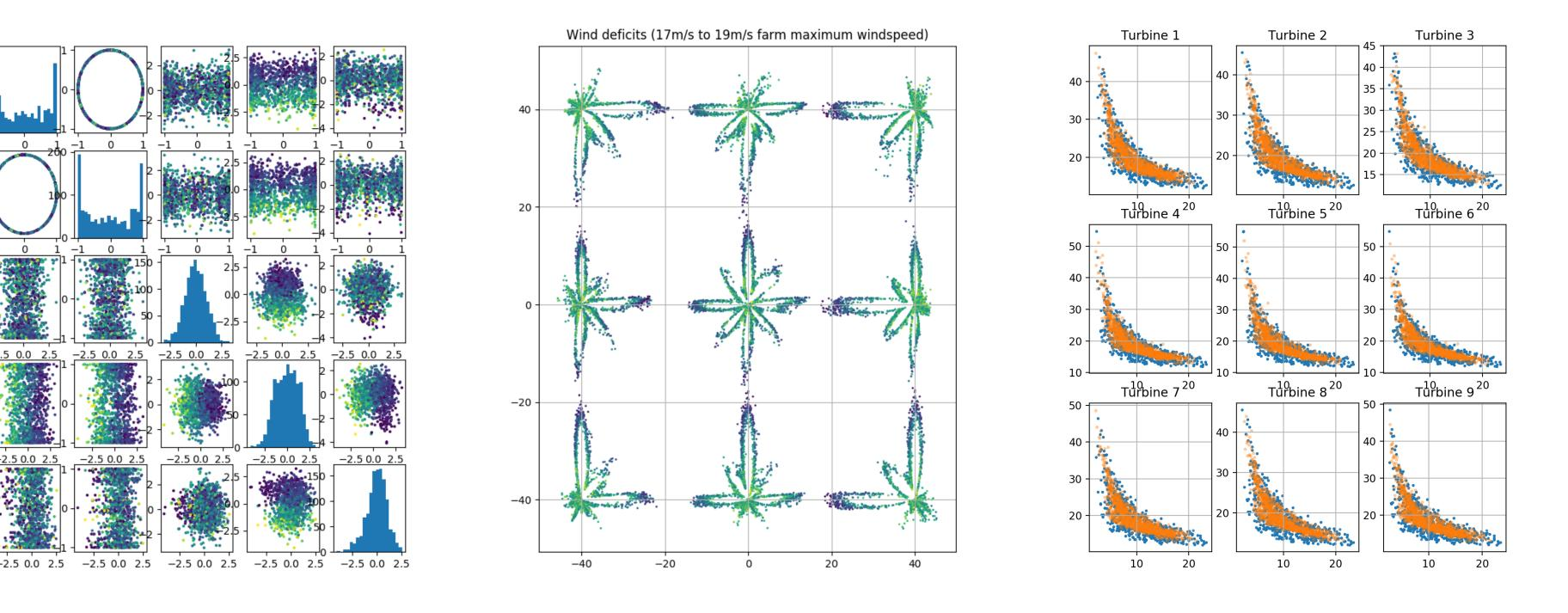
Left: Learned latent space, colored by farm-mean wind speed. Middle: Per-turbine visualization of samples from the learned distribution of wind deficits (marginalized w.r.t. wind-orientation and conditioned on a range of mean farm wind speeds) **Right**: Simulated (blue) and VAE-sampled (orange) joint distribution of 10-minute mean wind speed [m/s] turbulence intensity[-].
