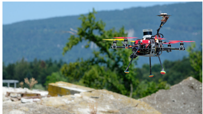
Fig. 5: A hexacopter MAV flying through a search and rescue training area (Sec. VIII-B1). The platform was equipped with a 64 beam lidar (visible), monocular camera, time-synchronized IMU, and RTK-GNSS (used for trajectory evaluation only).
