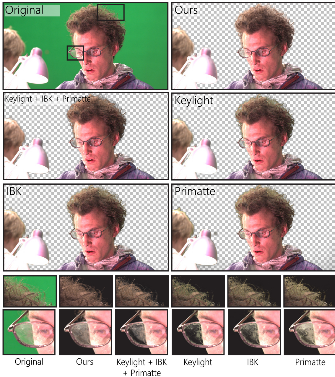
Figure 3.11.: Commercial keying tools, even when operated by a specialized compositing artist, may not be able to extract the fine details near intricate object boundaries while our algorithm is robust against such challenging regions.
