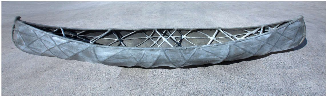
Figure 1: skeETHon, the four-metre-long canoe made entirely out of concrete.
