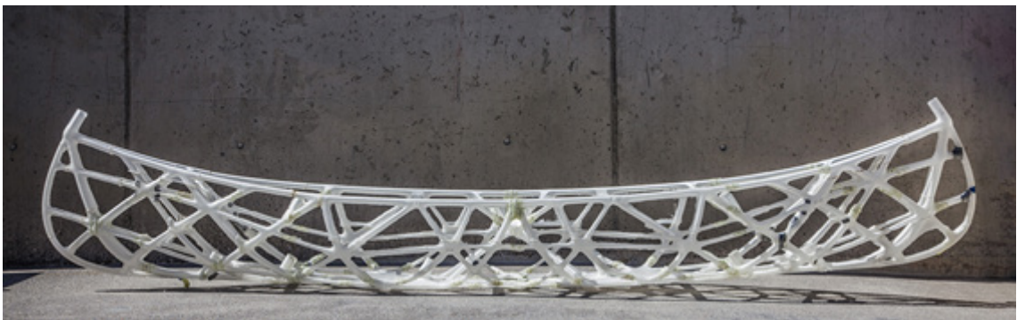
Figure 15: The 84 3D printed pieces assembled and ready for casting.
