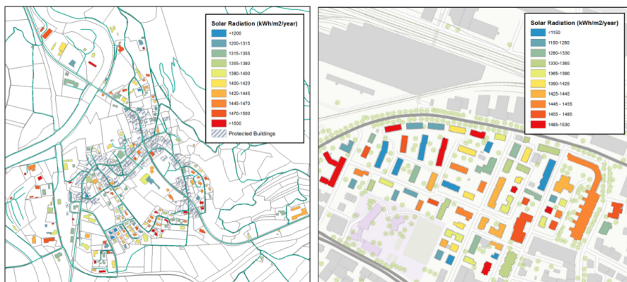
Figure 3.3.: Solar radiation potentials of the cases with Zernez on the left and Altstetten on the right.
