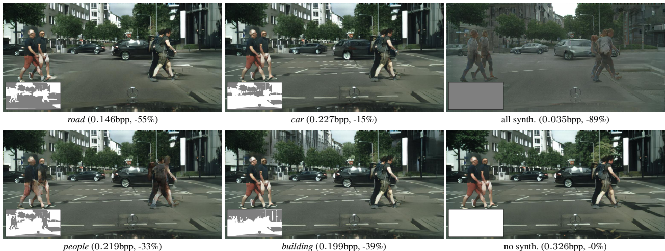
Figure 8. Synthesizing different classes using our SC network with C = 8 . In each image except for no synthesis , we additionally synthesize the classes vegetation , sky , sidewalk , ego vehicle , wall . The heatmaps in the lower left corners show the synthesized parts in gray. We show the bpp of each image as well as the relative savings due to the selective generation.
