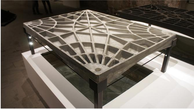
Figure 2: Exhibited physical prototype of the concrete rib-stiffened vaulted floor, supported on four corner supports and with representative steel ties.
