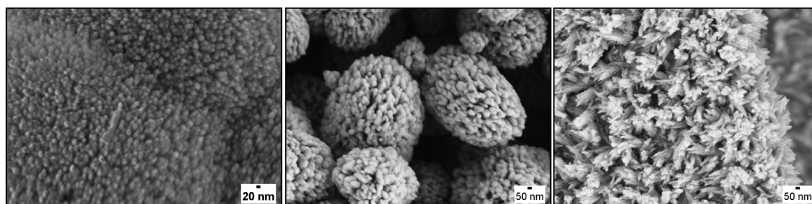
Figure C.1: SEM images displaying the primary particle sizes of ZnO agglomerates, nanovaterite agglomerates and hydroxyapatite platelets.
