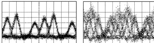
Fig. 7. Remaining  $3 \times 10$  Gbit/s (left) and  $7 \times 10$  Gbit/s (right) traces indicating pattern effects because of gain saturation after the strong control pulses (horizontal axis: 20 ps/div).
