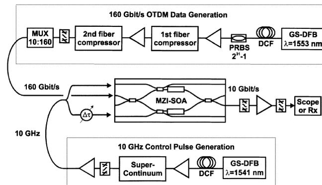
Fig. 4. Setup for the 160:10 Gbit/s demultiplexing experiment.
