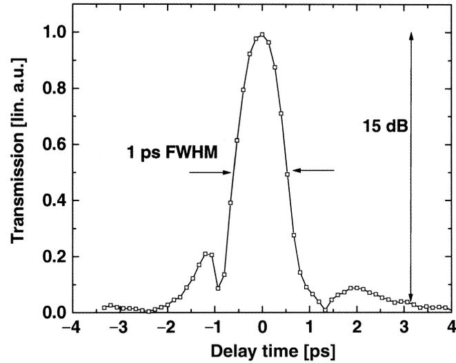
Fig. 3. Switching window measured with pump-probe technique (before deconvolution).
