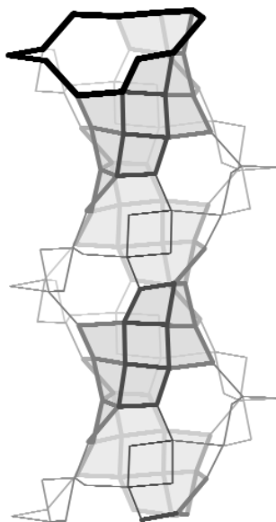
Fig. 6 The sinusoidal channel in chiral zincophosphate (IZA code CZP ) [16]. The distorted 12-ring defining the effective channel width and a chain showing the helical nature of the channel have been highlighted. Bridging oxygen atoms have been left out for clarity.
