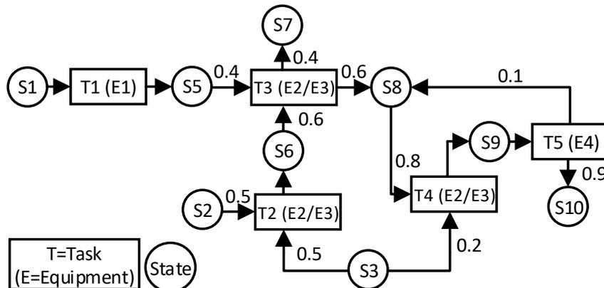
**Figure 3:** Batch production system of the case study from Kondili et al. [15]. For each task, we added demands of low- and high-temperature heating, cooling and electricity.
