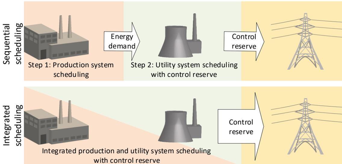
**Figure 1:** Sequential and integrated scheduling of production and utility system. In sequential scheduling, first, the production system is scheduled for the minimal production cost. Subsequently, the utility system is scheduled to provide the energy demand of the production system as well as control reserve to the grid. The integrated scheduling considers the production and utility system simultaneously.
