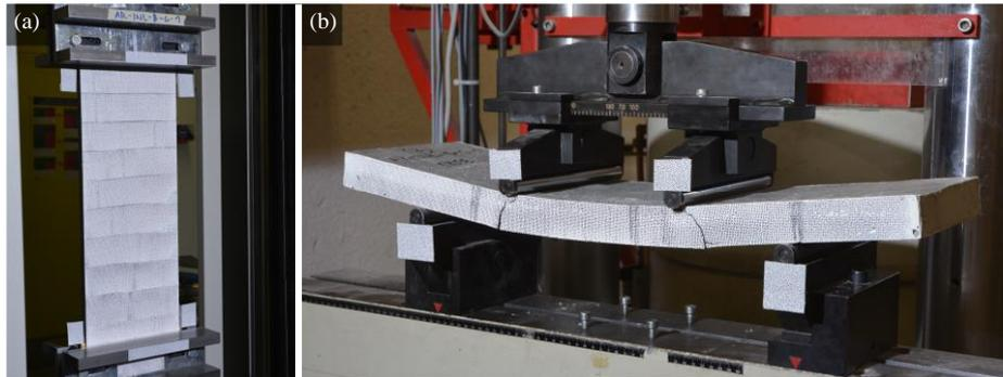
**Figure 7.** Textile reinforced concrete specimens (a) in uniaxial tension and (b) in bending.
