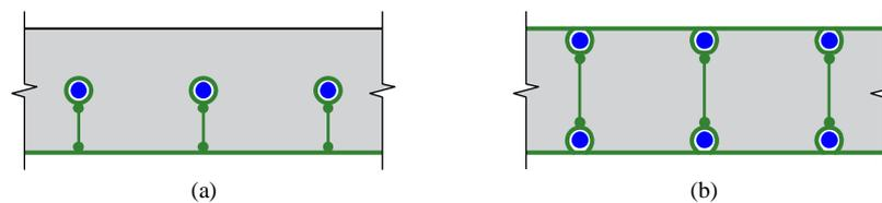
**Figure 6.** Concepts for integrating linear reinforcement into knitted formwork: (a) bottom layer suspended from reinforcement and (b) sandwich-elements with top and bottom layer.
