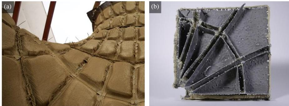
**Figure 3.** Ribbed cross sections from (a) inflating hollow pockets and (b) folding.
