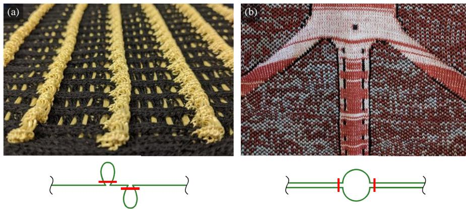
**Figure 1.** Weft-knitted textiles with (a) ribs and (b) channels.
