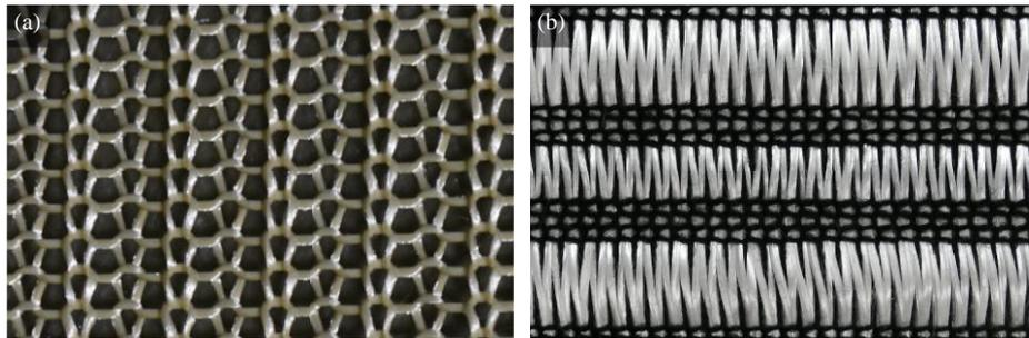
**Figure 4.** Flat weft-knitted textile with (a) aramid yarn and (b) glass fibre inlays (white rovings) within base pattern made out of acrylic yarn.
