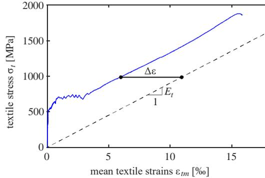
**Figure 8.** Load-deformation behaviour of tension ties with textile reinforcement.
