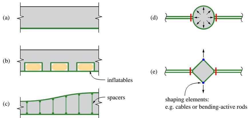
**Figure 2.** Schematic overview of possible cross sections with flexible formwork.
