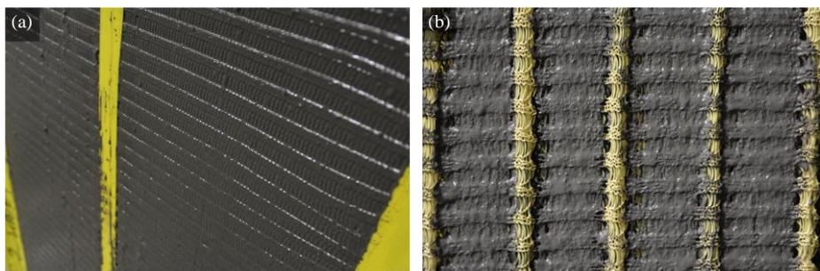
**Figure 5.** Knitted textile after application of cement paste coating (fresh state): (a) flat textile; (b) textile with ribs for bond enhancement.
