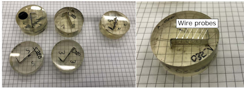
Figure 5.1: Epoxy probes each containing six wire cross-section samples.
