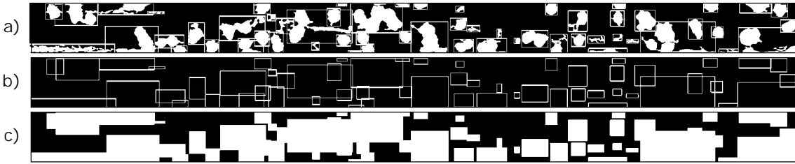
Figure 4.26: (a, b) Bounding boxes plotted around surface elements at their maximum points along and orthogonal to the wire length. Frames around the elements (c) Superposed bounding box areas.
