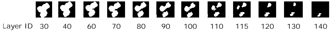
Figure 4.32: Horizontal cross-sections of the same cluster structure at different heights from Layer 30 to Layer 140. Grain peaks points in the cluster structure can be identified.
