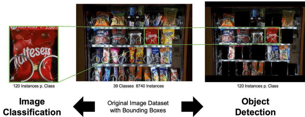
Fig. 5. Generation of training data with k images per product class for training the neural networks in the image classification and object detection tasks.
