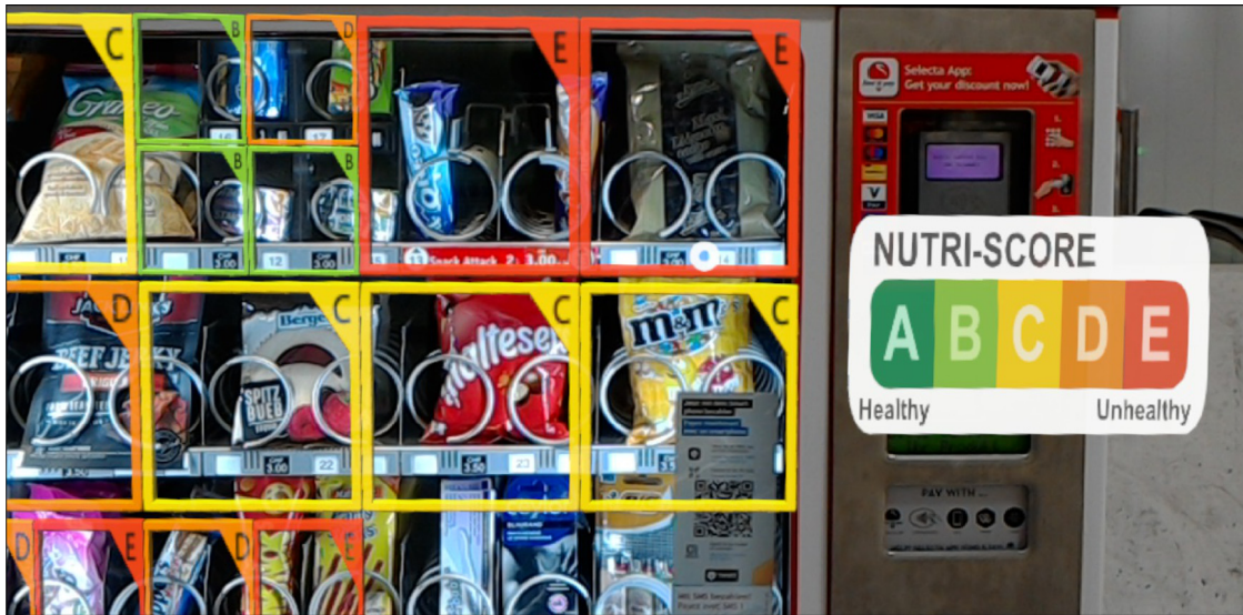
Fig. 6. Computer-vision on packaged products allows novel human-object interactions, e.g. passively triggered diet interventions in the absence of markers or barcodes (Screenshot of Microsoft HoloLens viewing the study’s vending machine).
