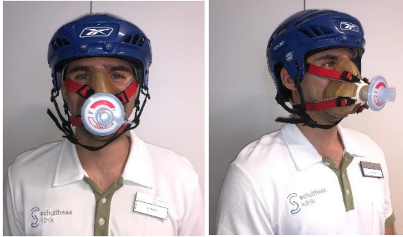
Figure 7: Pictures of the assembled prototype how it should be worn with the helmet
