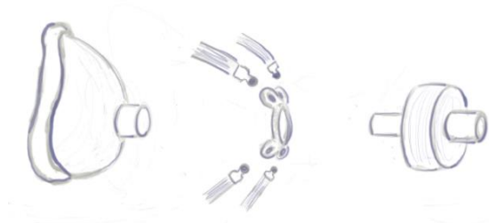
Figure 3: Prototype components: A simple mask is combined with a filter and hold to the head with a mount and straps.
